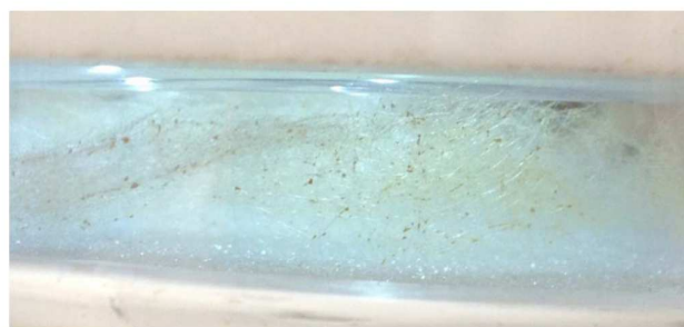
Figure 9. Expanded Quartzel ® inside the reactor after irradiation in the presence of toluene for 500 min.
