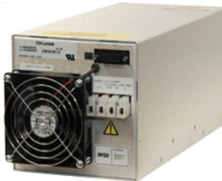
Figure 6.2 HV charging power supply [6.1]
