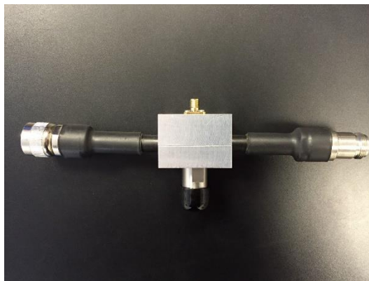
Figure 5.18 Multi-GHz coaxial cable arrangement
