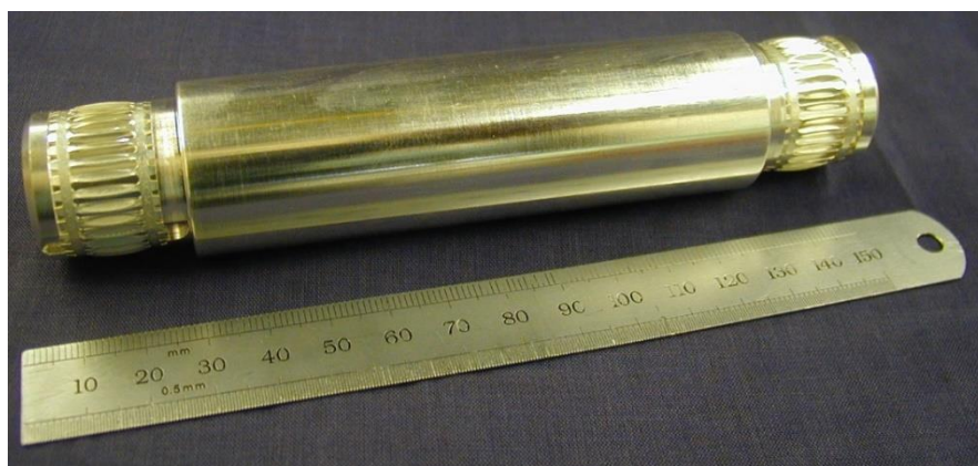
Figure 6.11 HV electrode bar of spark gap
