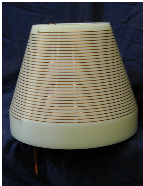
Figure 2.5 Secondary winding of Tesla transformer
