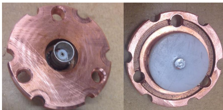
Figure 5.3 Voltage sensor for oil-filled Blumlein PFL
