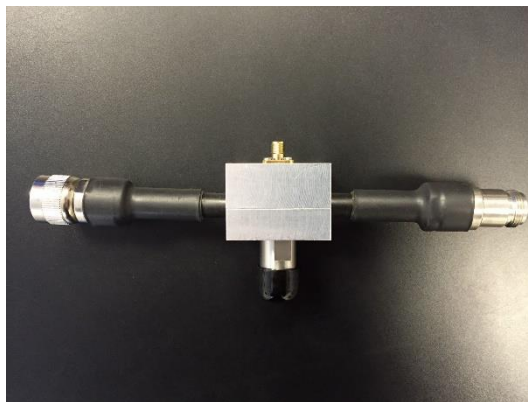
Figure 5.18 Multi-GHz coaxial cable arrangement
