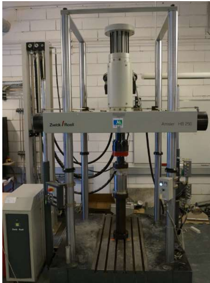
Figure 3.3. Zwick /Roell Amsler HB250 press and compaction mould
