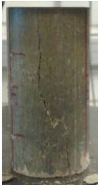
Figure 5.6. Typical compressive failure mechanism (sample S10 - CS50 - W5.6 - see Table 3.3)
