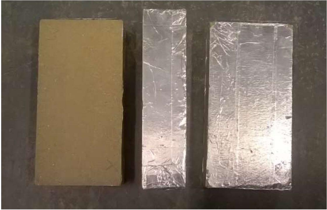
Figure 6.9. View of the three earth bricks before testing: unsealed surface (200x100 mm 2 ) and two of the five sealed surfaces (200x50 mm 2 and 200x100 mm 2 )
