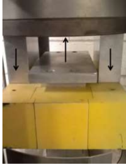
Figure 3.12. Brick demoulding phase
