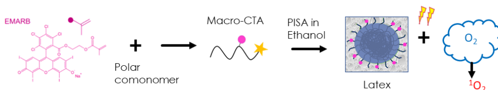
Figure 1 – principle of photoactive polymer colloids synthesis
