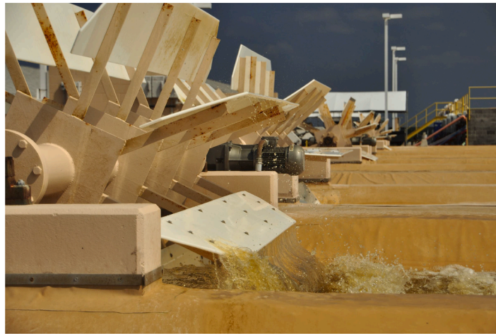
Fig. 3. Conventional 8-Blade Flat Paddlewheel Configuration. Cellana's Kona Demonstration Facility (KDF) on the Big Island of Hawaii.
