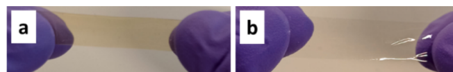
Fig. 5. Photos of a) 100% CS testing samples and b) CS/SiO 2 hybrid containing 90 wt% of TEOS.
