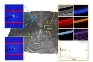
**Figure 1**: Combination of techniques, e.g micro-CT, SAXS and SEM-EDX, for the structural and composition analysis of a teleost fish scale - *Salmo salar*: 3D image is from micro-CT; (A) and (B) locate two X-ray spots, anterior and posterior scale areas, with the corresponding SAXS patterns, respectively, where the X-ray beam hit for SAXS analysis; (C) is a cross section of the anterior area observed with SEM-EDX, where the bi-layer structure collagen/mineral is visible.
