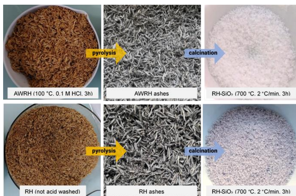
Figure 4. Pictures of the effect of acid pretreatment of RH through pyrolysis and calcination processes.
