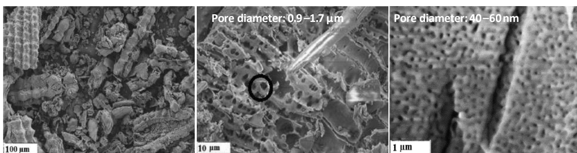
Figure 7. SEM pictures of acid-treated SiO 2 from RH.
