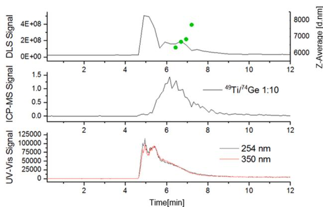
Fig. 5. Fractograms of cycle 7 (centrifuged at 3  $\mu$ m) recorded by different detectors: DLS (size information), ICP-MS (composition) and UV-Vis. The green dots correspond to the hydrodynamic diameter determined by AF4-DLS.
