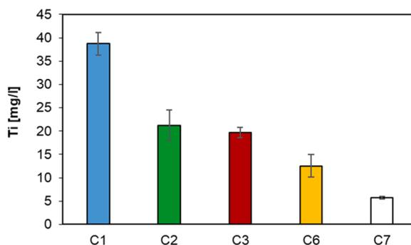
Fig. 4. Ti concentration (mg/L) after TiO<sub>2</sub>/UV-vis photocatalysis.
