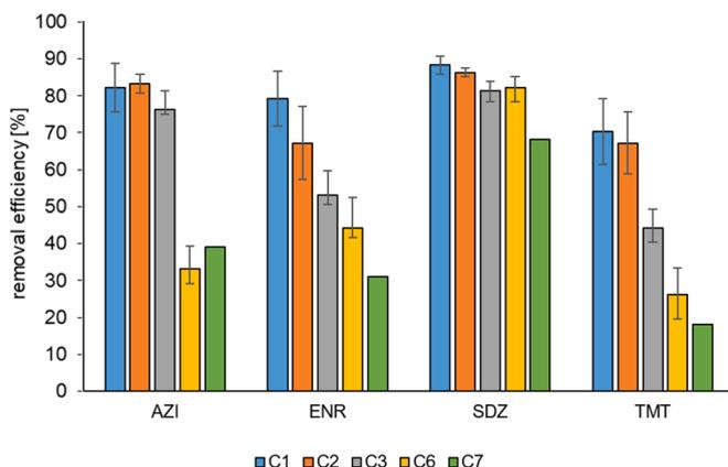
Fig. 3. Antibiotic removal applying TiO<sub>2</sub>/UV-vis photocatalysis to antibiotic-fortified WWTP effluent during 7 cycles.
