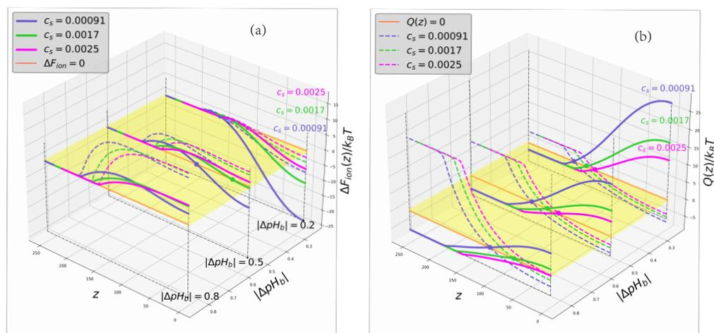
**Figure 4.** Cross-sections of the 2D profiles of the insertion free energy  $\Delta F_{ion}(z, |\Delta pH_b|)$  (a) and BSA globule charge  $Q(z, |\Delta pH_b|)$  (b) for the cases of polyanionic (solid curves,  $pH_b > pI$ ) and polycationic (dashed curves,  $pH_b < pI$ ) brushes. The color code corresponding to different salt concentrations  $C_s$  is indicated at the curves. Colored circles in the panel correspond to the charge inversion points  $z = z^*$ .
