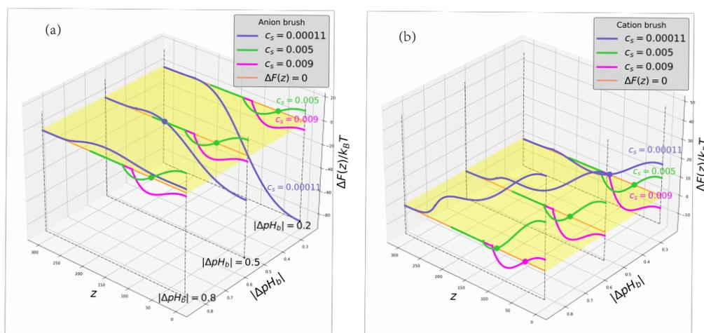
**Figure 7.** Cross-sections of the 2D profiles of the BSA insertion free energy  $\Delta F(z, |\Delta pH_b|)$ , for the cases of polyanionic,  $pH_b > pI$  (a) and polycationic,  $pH_b < pI$  (b) brushes. The color code corresponding to different salt concentrations  $C_s$  is indicated in the legend and at the curves. Colored circles correspond to the points of vanishing  $\Delta F(z)$ .
