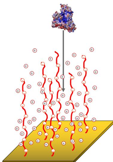
**Figure 2.** Schematics of the BSA globule insertion into the polyanionic brush. Mobile counterions (cations) are shown explicitly. Blue, red and white patches on the globule surface correspond to anionic, cationic and neutral residues, respectively.
