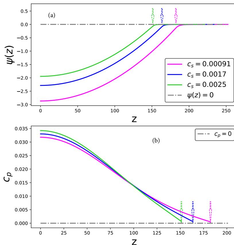
**Figure 8.** Electrostatic potential of the polyanionic brush (a) and the distribution of the monomer  $c_p(z)$  density  $c_p(z)$  inside the brush (b) as a function of the distance from the grafting surface  $z$  and varied salt concentration  $C_s \equiv c_s a^3$  for  $\mathcal{N} = 300$ ,  $s/a^2 = 100$ . The brush boundary,  $z = H$ , is indicated by the arrows.
