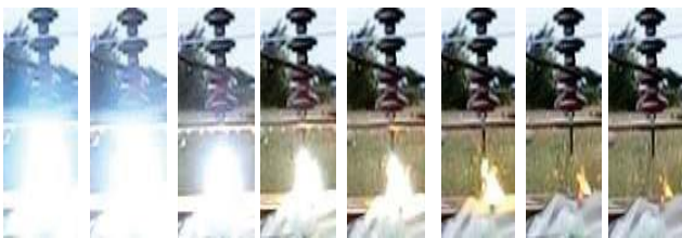
Figure 10. Dynamics of diode plasma during a high energy shot (stills from a 1000 fps movie)
