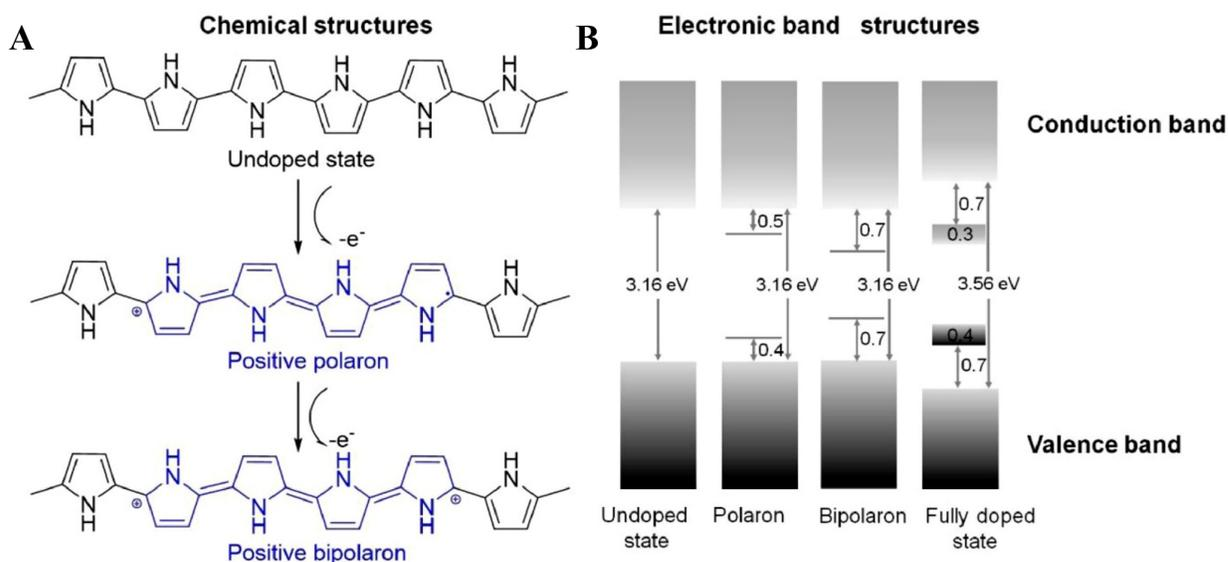
**Figure 7.** (A) Chemical and (B) Electronic band structures of PPy in different doping states. Adapted with permission from Ref.<sup>142</sup>. Copyright© 2021 Elsevier Ltd.
