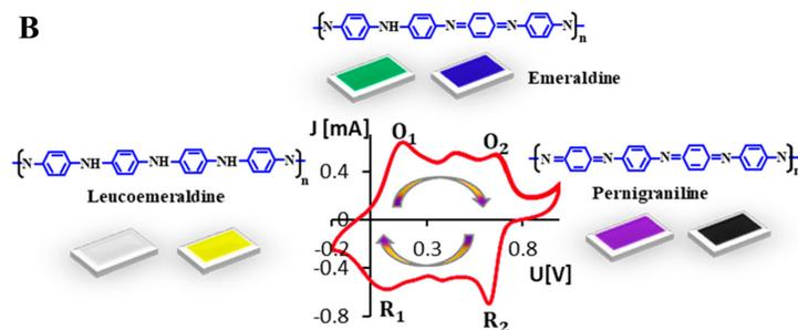
**Figure 5.** (A) Different redox/protonation states of PANI and their corresponding colors. Adapted with permission under a Creative Commons (CC-BY 4.0) from Ref.<sup>90</sup>. Copyright © 2017 MDPI. (B) Another view of PANI states and color switching during cyclic voltammetry experiment. Adapted with permission from Ref.<sup>18</sup>. Copyright© 2019 American Chemical Society.
