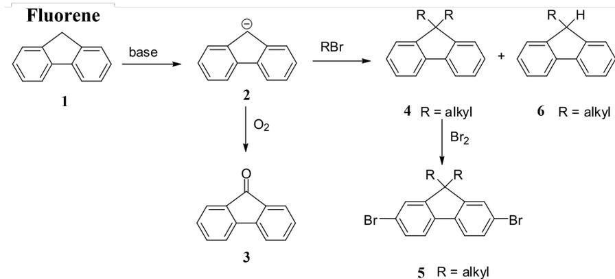
**Figure 11.** Alkylation of fluorene to produce monomers for PDAFs. (4 and 5 can be used as PDAFs' precursors). Adapted with permission from Ref.<sup>248</sup> Copyright © 2008, Springer-Verlag Berlin Heidelberg.
