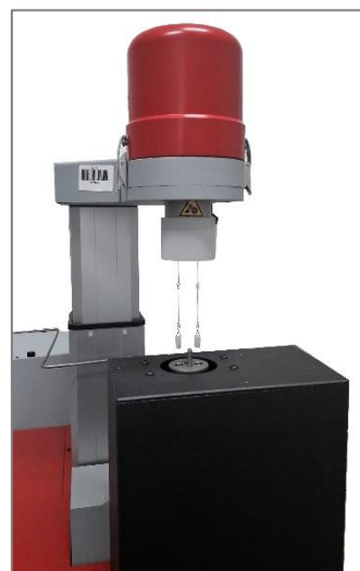
Figure 3b. Introduction of the two crucibles in the columns.
