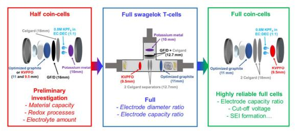
**Figure 1**. Schematic representation of the approach followed in this work to optimize the assembly of highly reliable K-ion full coin cells.
