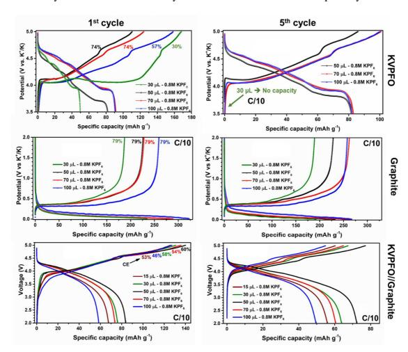
**Figure 2**. Galvanostatic profiles during the 1<sup>st</sup> and 5<sup>th</sup> cycles at C/10 for KVPO<sub>4</sub>F<sub>0.5</sub>O<sub>0.5</sub>//K cells (between 3.5-5 V), graphite//K cells (between 2-0.01 V) and KVPFO//graphite cells (between 2-5 V with both negative/positive diameter and capacity ratios of 1.16) as function of the 0.8M KPF<sub>6</sub> EC:DEC electrolyte volume as indicated.
