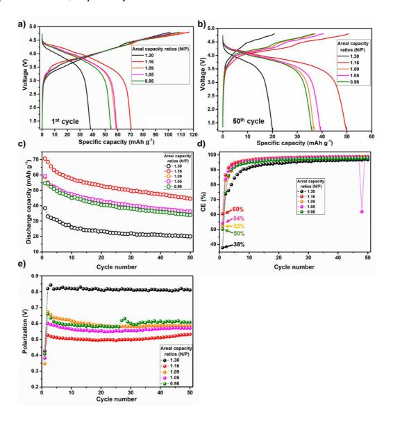
**Figure 4**. a) 1<sup>st</sup> and b) 50<sup>th</sup> galvanostatic cycles profiles between 1.2-4.8 V at C/10 for KVPFO//graphite full coin-cells as function of the capacity ratio. c) Capacity retention, d) coulombic efficiency and e) polarization for the same cells over 50 cycles. The graphite/KVPFO diameter ratio was here fixed to 1.16. Note that the reported capacities were calculated based on KVPFO weight.
