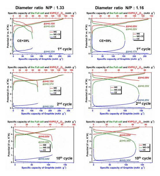
**Figure 3**. Galvanostatic profiles during the 1<sup>st</sup>, the 2<sup>nd</sup> and 10<sup>th</sup> cycles at C/10 between 3.5-5 V for KVPFO//graphite 3-electrodes T-cells with N/P diameter ratio of 12.7/9.5 = 1.33 and 11/9.5 = 1.16. The graphite/KVPFO capacity ratio was here fixed to 1.16. Note that  $\Delta V$  corresponds to the polarization, *i.e.* the difference between the average potentials.
