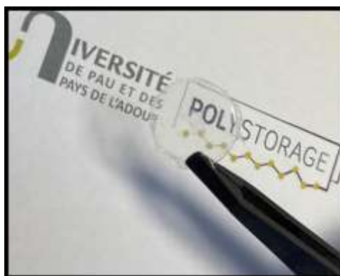
Figure S16: Exemplary pictures of self-standing transparent films ( \varnothing 16 mm, L= 100 \mu\text{m} ) derived from block copolymer electrolyte sc\text{-(A}_{0.62}\text{)}_{0.80}\text{B}_{0.20} .
