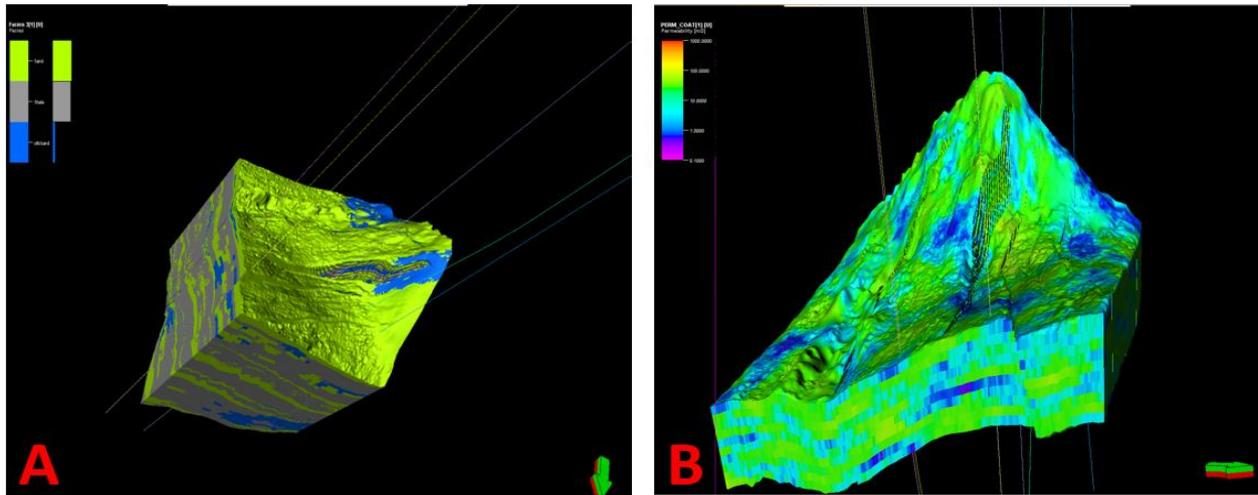
Figure 6. 3D Grid showing (A) facies distribution and (B) Porosity distribution
