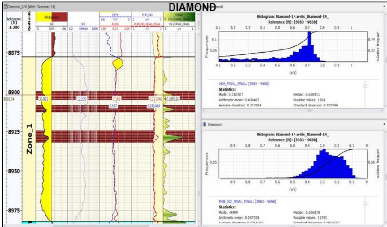
Figure 10. Result of the shale volume and effective porosity curves generated for well Diamond
