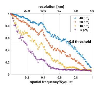
**Figure 4.** Spatial resolution estimation by Fourier ring correlation (FRC) method. Estimation of spatial resolution for tomograms reconstructed by MLEM from different numbers of projections chosen from the measured 360 angular projection dataset. The fixed 0.5 threshold was used for FRC analysis. The Nyquist frequency is  $0.25 \, \mu m^{-1}$ .
