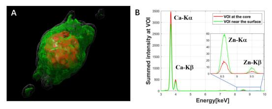
**Figure 7.** Extraction of the mean XRF spectra within the volume of interest of the reconstructed calcification micro-sphere shown in Fig. 5D,E. (**A**) Reconstructed result by MLEM algorithm from the total intensity of the XRF spectra, grey volume: reconstructed total sphere volume, red and green volumes: core and surface rim regions, respectively. (**B**) Comparison of the mean XRF spectra of the core (red) and surface rim (green) volumes.
