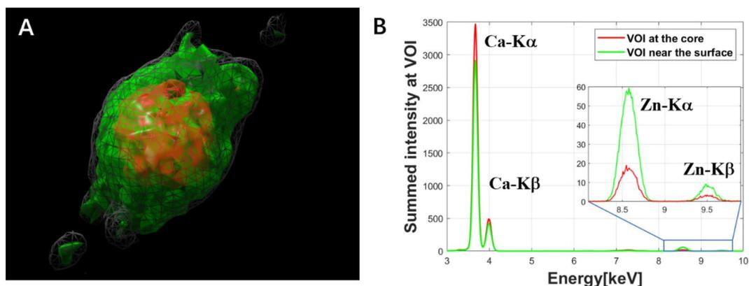
**Figure 7.** Extraction of the mean XRF spectra within the volume of interest of the reconstructed calcification micro-sphere shown in Fig. 5D,E. **(A)** Reconstructed result by MLEM algorithm from the total intensity of the XRF spectra, grey volume: reconstructed total sphere volume, red and green volumes: core and surface rim regions, respectively. **(B)** Comparison of the mean XRF spectra of the core (red) and surface rim (green) volumes.
