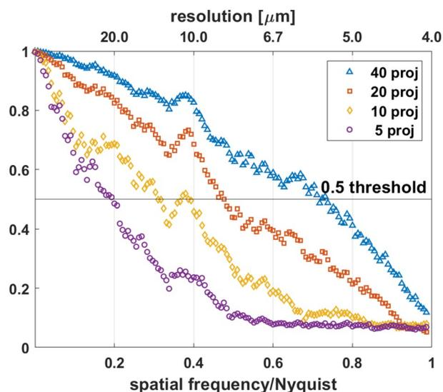
**Figure 4.** Spatial resolution estimation by Fourier ring correlation (FRC) method. Estimation of spatial resolution for tomograms reconstructed by MLEM from different numbers of projections chosen from the measured 360 angular projection dataset. The fixed 0.5 threshold was used for FRC analysis. The Nyquist frequency is  $0.25 \mu\text{m}^{-1}$ .
