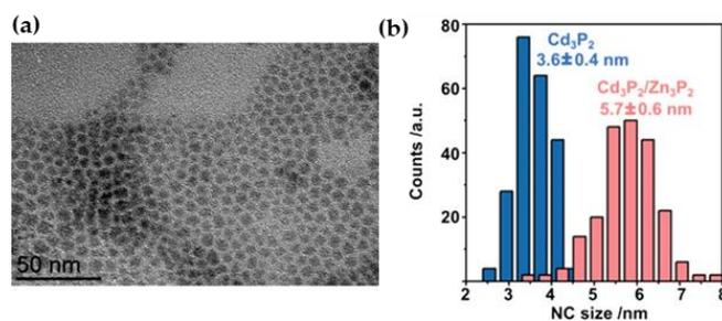
**Figure 1.** (a) TEM image of Cd<sub>3</sub>P<sub>2</sub>/Zn<sub>3</sub>P<sub>2</sub> core-shell NCs. (b) Histograms of measured NC sizes for Cd<sub>3</sub>P<sub>2</sub> cores and Cd<sub>3</sub>P<sub>2</sub>/Zn<sub>3</sub>P<sub>2</sub> core-shell NCs.
