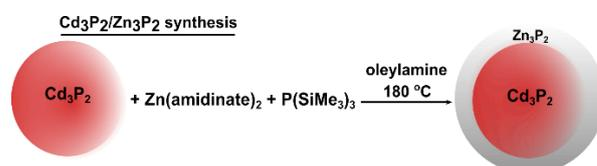
**Scheme 1.** Scheme detailing the synthesis of a  $\text{Zn}_3\text{P}_2$  shell on top of  $\text{Cd}_3\text{P}_2$  cores.
