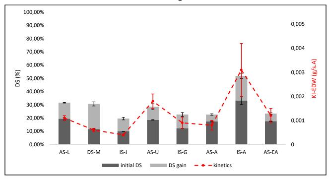
Figure 3: EDW tests performance for different sludges (final DS and dewatering kinetics) In the following Table 4, the obtained values are listed.
