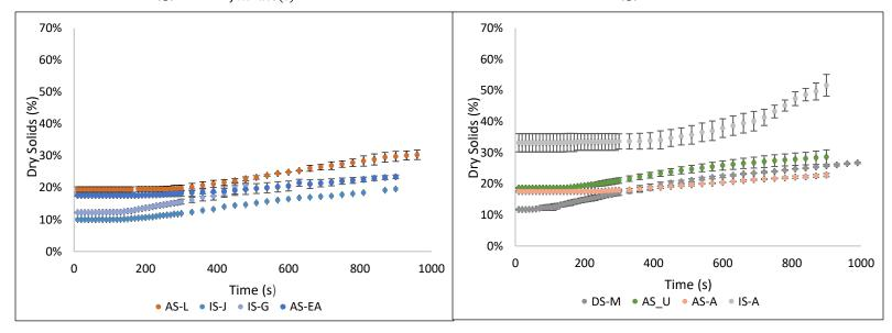
Figure 2: evolution of dry solids content over time during electrodewatering tests
