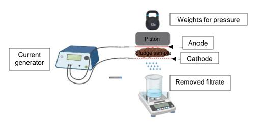
Figure 1: experimental setup
