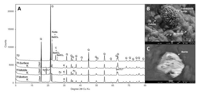
Fig. 8 Powder XRD patterns for the solid phase (A) before incubation ( $t_0$ ) and after 87 days of incubation in the reactor ( $t_f$ ). SEM images of the solid phase at  $t_f$  (B) and (C). XRD patterns at  $t_f$  were collected at the surface of the reactor ( $t_f$ -surface), at mid-height ( $t_f$ -middle) and at the bottom ( $t_f$ -bottom). K: kaolinite, Q: quartz, C: calcite, Py: pyrite. The peak labelled 'clays' originated from (020) and (110) of clay minerals.
