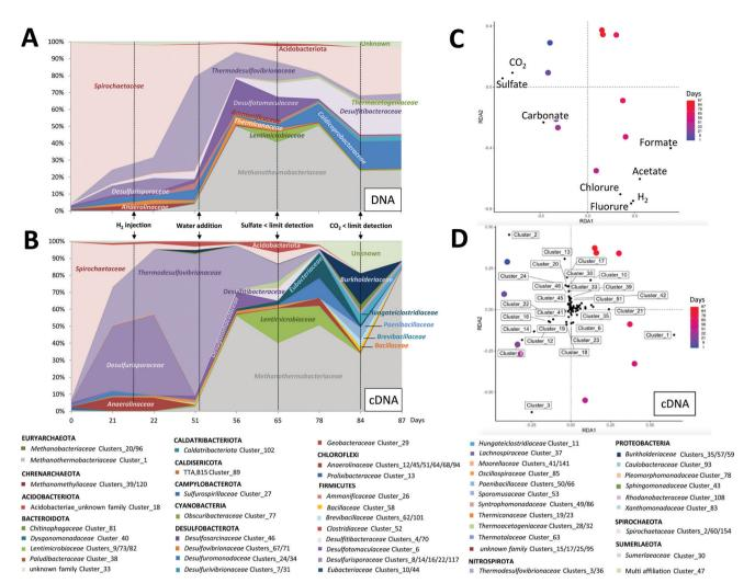
Fig. 5 Evolution of the microbial community during the incubation at 47  $^{\circ}$ C, at 85 bar (CH<sub>4</sub>, 1% CO<sub>2</sub>) before and after hydrogen injection (95 bar with 10% H<sub>2</sub>). The taxonomic diversity is monitored by 16S rRNA gene sequencing performed in an aqueous phase sampled from the reactor throughout the experiment.
