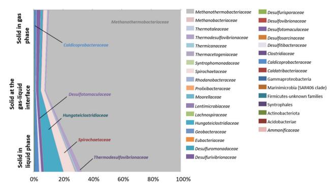
Fig. 7 Microbial community after the incubation at 47 °C, at 85 bar (CH<sub>4</sub>, 1% CO<sub>2</sub>) followed by hydrogen injection (95 bar with 10% H<sub>2</sub>). The taxonomic diversity was monitored by 16S rRNA gene sequencing performed on different heights of the solid phase at the end of the experiment.
