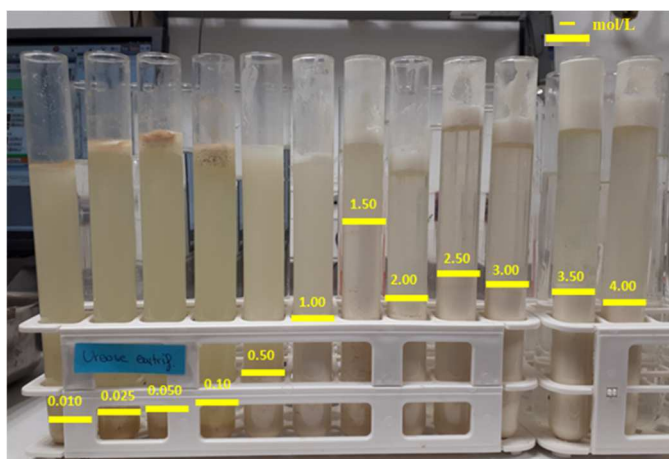
317 318 Fig. 7: Visual inspection of test-tubes 72 hours after adding calcium chloride (equimolar urea and calcium 319 chloride concentrations varying from 0.010 mol/L to 4 mol/L).
