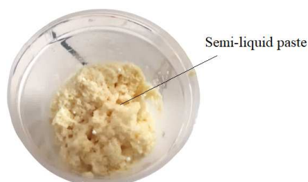
346 Fig. 9: Formation of a semi-liquid paste after addition of calcium chloride to test-tubes containing distilled water, 347 soybeans fine powder and urea (urea/calcium chloride concentration of 2.50 mol/L).
