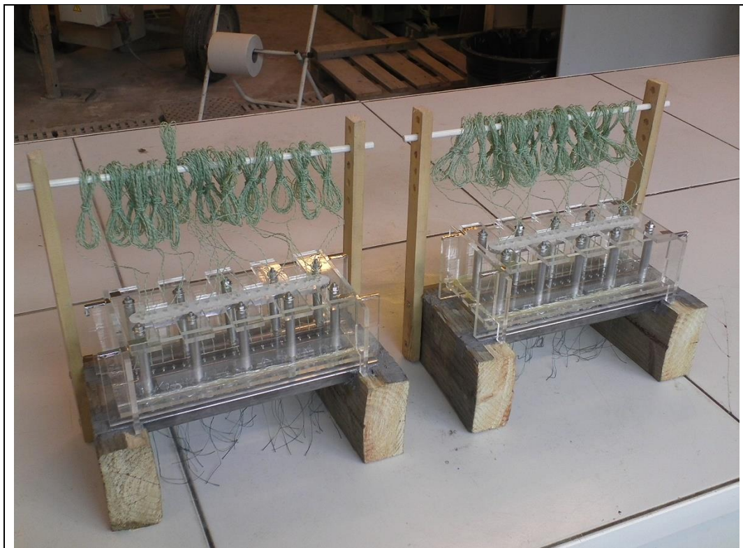
A pair of assembled moulds ready for concrete to be poured.
