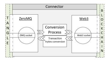
Fig. 4. Connector's Architecture
