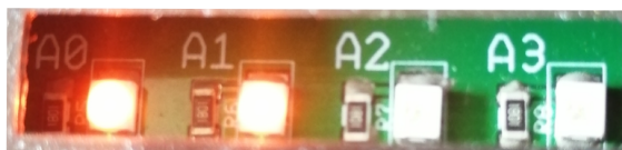
Figure 13: 4 LEDs on the motherboard indicate the selected plug.
