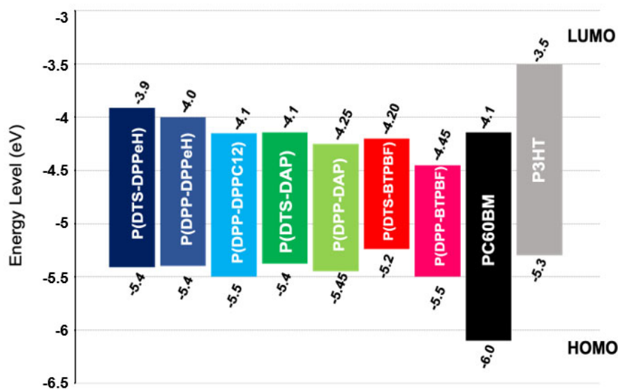
Figure 5. HOMO-LUMO energy levels of the copolymers (A-A') based on DPP and (D-A) based on DTS determined by cyclic voltammetry.
