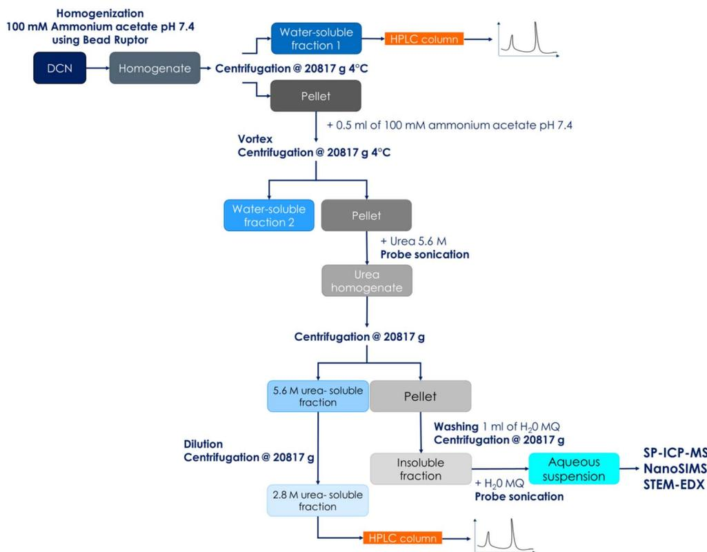
FIGURE 1. Sample preparation procedure and resulting fractions.
