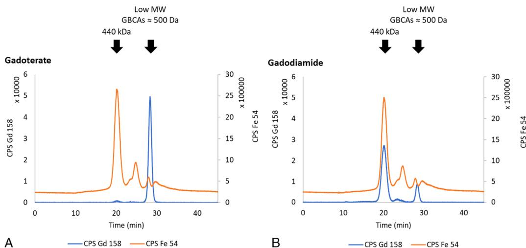
**FIGURE 4.** SEC-ICP-MS  $^{158}\text{Gd}$  and  $^{54}\text{Fe}$  chromatograms of water-soluble fraction of the DCN from the animals treated with gadoterate (A) or gadodiamide (B). MW indicates molecular weight. CPS, counts per second.
