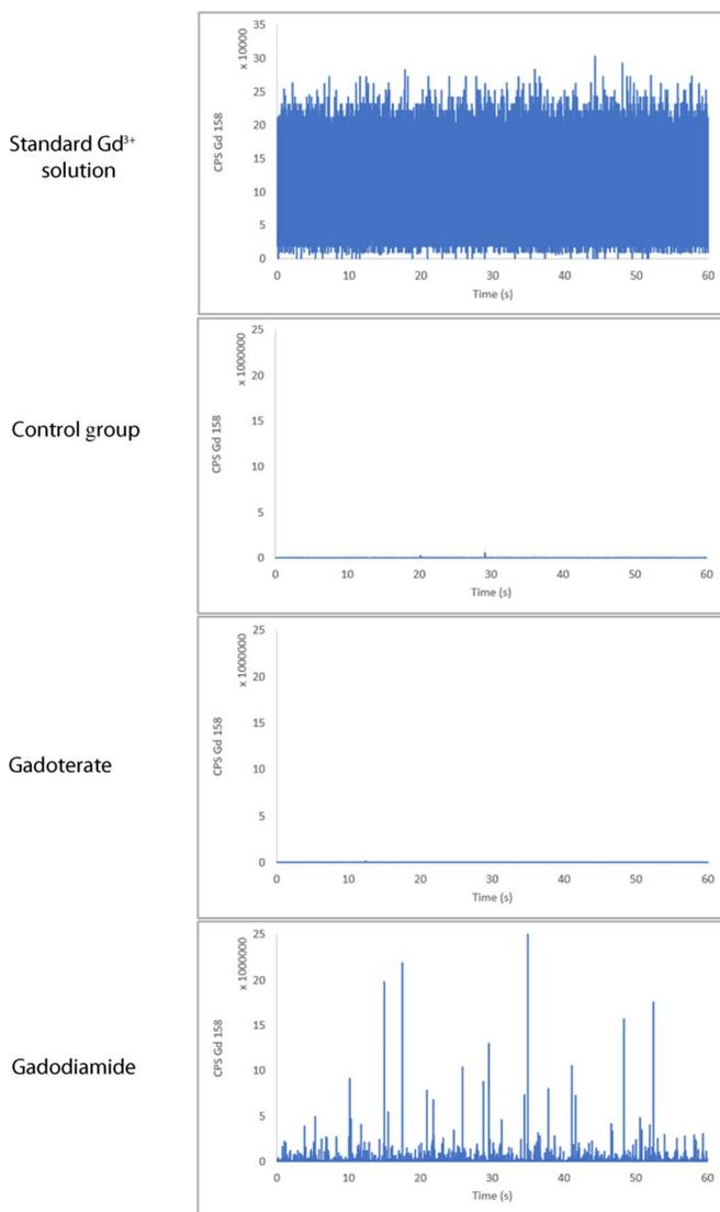
**FIGURE 5.** SP-ICP-MS  $^{158}\text{Gd}$  time scans obtained for ionic  $\text{Gd}^{3+}$  standard and for the aqueous suspension of final insoluble residue of DCN from the control, gadoterate, and gadodiamide treated groups.
