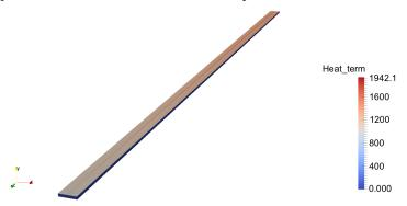
**Figure 14.** Heat- generation source (in W/m<sup>3</sup>) for  $\omega_1 = 2.45$  GHz and the incident electric field polarized in the direction of the fibers.
