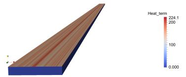
**Figure 13.** Heat-generation source (in W/m<sup>3</sup>) for  $\omega_1 = 2.45$  GHz and the incident electric field polarized in the normal direction with respect to the fiber orientation.
