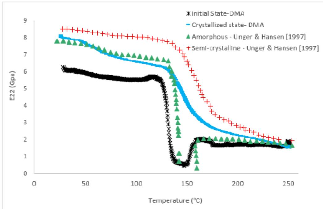
Figure 1 - Transverse modulus for the material obtained with DMA and compared with results from [7]
