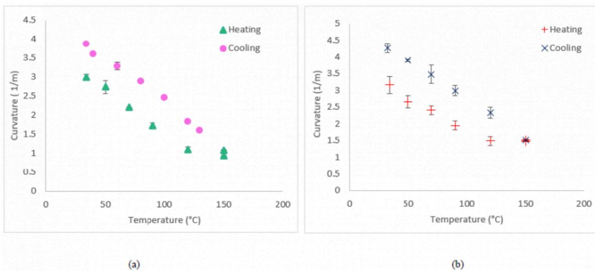
**Figure 4 - Evolution of the measured curvature with temperature for [90<sub>3</sub>/0<sub>3</sub>] manufactured with (a) cold mandrel and (b) hot mandrel**
