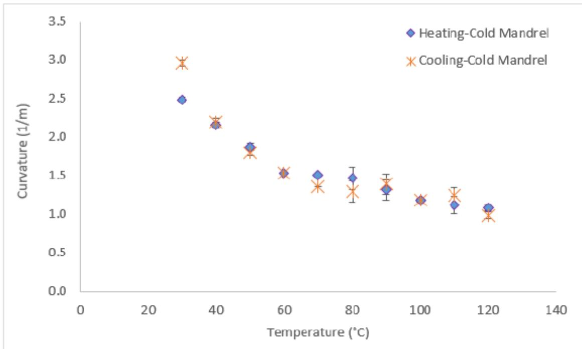
Figure 3 - Evolution of the measured curvature with temperature for [90<sub>3</sub>/0<sub>3</sub>] manufactured with cold mandrel
