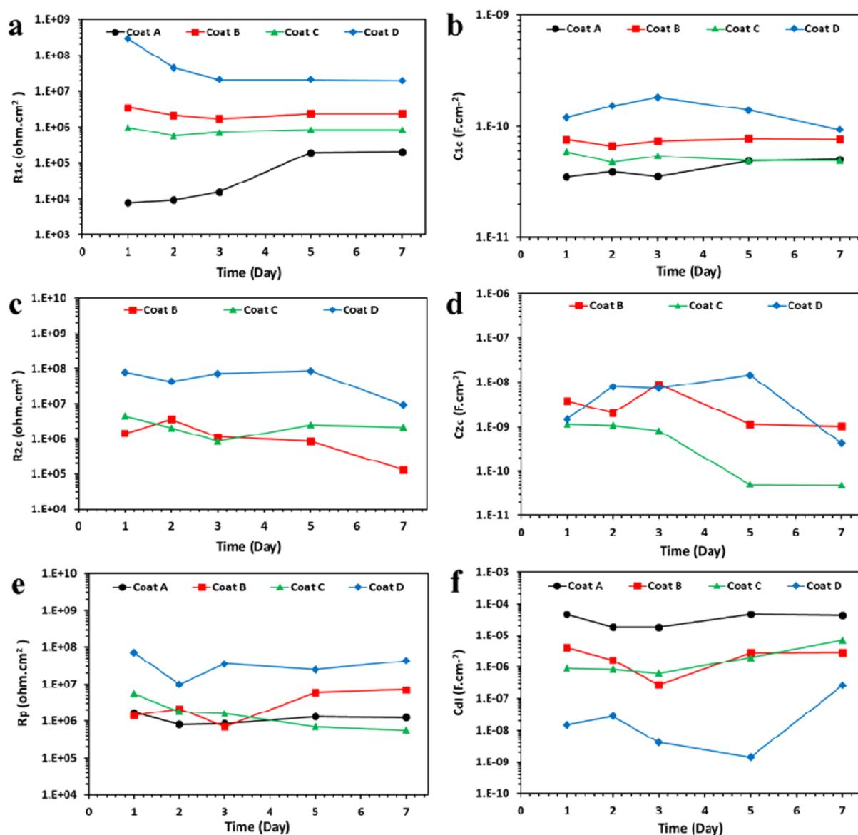
**Figure 7.** EIS results of the artificially scratched coatings during the immersion period: (a)  $R_{1C}$ , (b)  $C_{1C}$ , (c)  $R_{2C}$ , (d)  $C_{2C}$ , (e)  $R_p$  and (f)  $C_{dl}$ .
