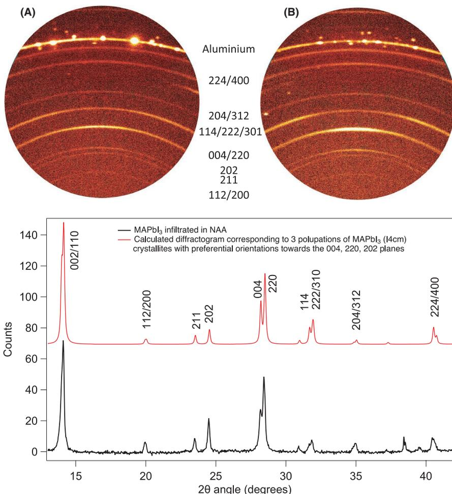
**FIGURE 5** 2D area images of grazing incidence XRD of the MAPbI<sub>3</sub> layer deposited on bare aluminum substrates (A) and infiltrated in NAA layers (B). The Debye rings are indexed with the diffraction planes
