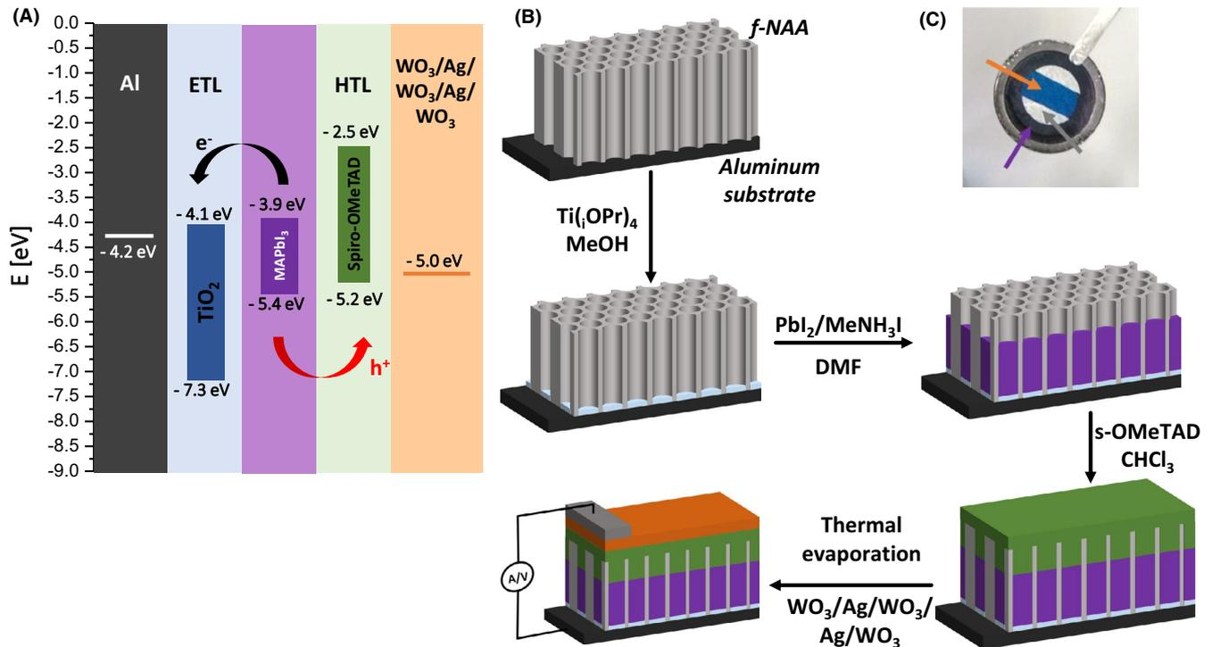
**FIGURE 1** A, Band diagram of the NAA-PSC device fabricated in this study; (B) schematic depiction of the solar cell device fabrication; (C) picture of an actual device, the purple arrow points to the MAPbI<sub>3</sub> layer, the orange arrow points to the semitransparent anode, while the gray arrow points to the silver upper contact
