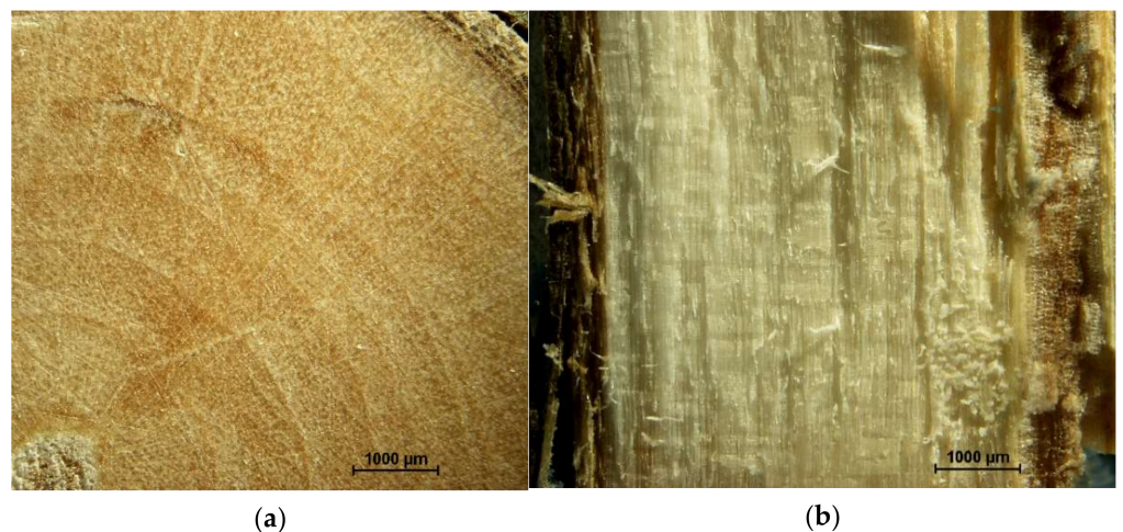
Figure 3. Cross-cut: (a) across and (b) along the fiber of the chokeberry stalk.
