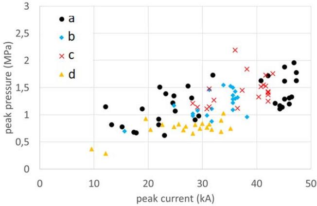
Fig. 8. Peak pressures as a function of peak current. The results were obtained using generator No.2 with the pairs of electrodes presented in Fig. 6 and Table II, mounted at a distance  $d = 5$  mm apart.
