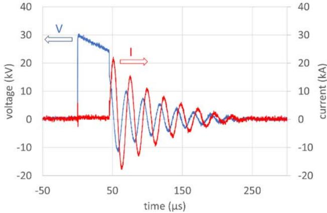
Fig. 2. Typical voltage and current waveforms recorded during a shot using generator No.2, with the capacitor initially charged to  $V_0 = 30$  kV and with the distance between the electrodes  $d = 4.8$  mm. The breakdown takes place at  $t_b = 45$   $\mu$ s, when the voltage is only  $V_b = 23.5$  kV.
