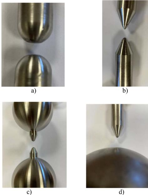
Fig. 6. Photographs of the various electrode pairs used in the preliminary studies. (a), (b), (c) and (d) correspond to the pairs (a), (b), (c) and (d) described in Table II.
