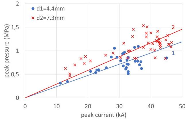
Fig. 11. Variation in the peak pressure for various peak currents flowing through the spark gap corresponding to two inter-gap distances with a constant measurement distance  $r = 820$  mm. The lines obtained by the least-square fit method (Pearson's correlation coefficients: 0.982 and 0.978, respectively) prove that the peak pressure is indeed proportional to  $(d)^{1/2}$  as predicted by (17).
