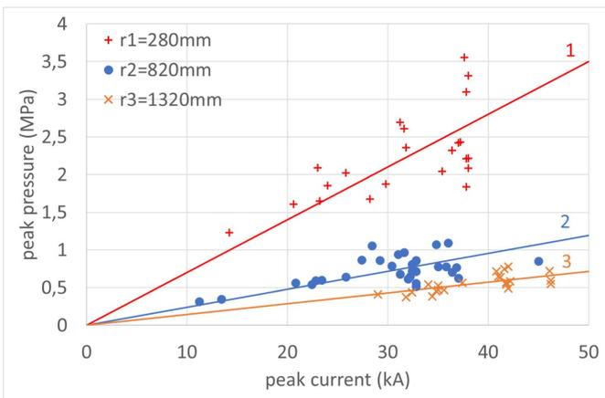
Fig. 10. Variation in the peak pressure for various peak currents flowing through the underwater spark with a constant inter-electrode distance  $d = 4.5$  mm. The lines obtained by the least-square fit method (Pearson's correlation coefficients: 0.982, 0.978, and 0.990, respectively) prove that the peak pressure is proportional to the inverse of the distance  $r$  between the hydrophone and the spark gap, as predicted by (17).
