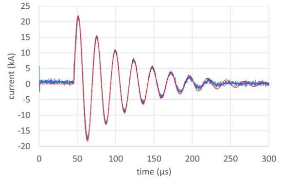
Fig. 3. Comparison between the experimental current waveform of Fig. 2 and the current calculated with (18), with  $R_{SD} = 10$  m $\Omega$ . As for obtaining a perfect fit (the theoretical prediction and the experimental data are indistinguishable), the term  $R_{SD}$  is not required to vary during the discharge, and the first hypothesis of the model is thus proven.
