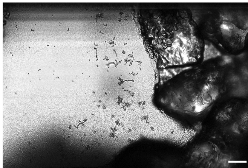
Figure 5. Methane hydrate halo and filaments on the floor of the glass cell on warming from -16 to -5\text{ }^{\circ}\text{C} in run 5. Scale bar: 50\text{ }\mu\text{m} .
