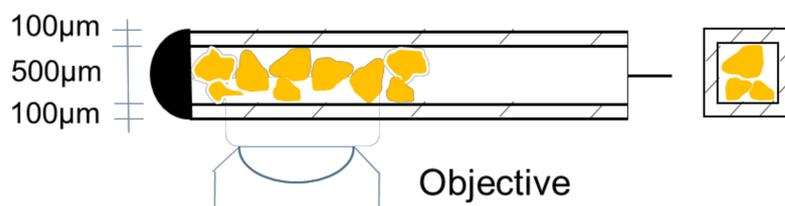
**Figure 1.** Experimental setup for optical microscopy runs. The cell, a thin glass capillary with a square cross-section, is inserted into a thermostated holder (not shown), on an inverted microscope.
