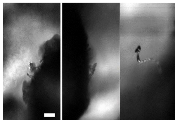
Figure 7. Examples of the shorter methane hydrate filaments growing from sand grains at 7\text{ MPa} , 2^\circ\text{C} in run 6. Scale bar: 20 \mu\text{m} .
