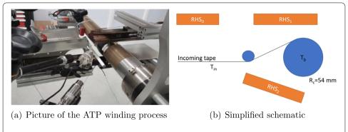
**Fig. 1** The ATP winding process with the three radiative heat sources marked as  $RHS_1$  and  $RHS_2$ , the incoming tape temperature is  $T_{in}$ , the cylindrical deposition base has a radius  $R_c = 54$  mm and a controlled temperature  $T_b$
