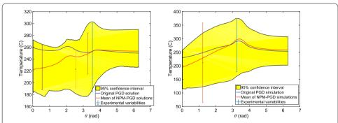
(a) Layer l-1 along with the temperature (b) Layer l along with the temperature measured by probes 1, 2, 3 and 4 illustrated sured by probes 1 and 2 illustrated in figure in figure 2(b) for set 2 of experimental pa-2(a) for set 2 of experimental parameters rameters
