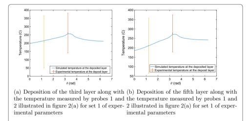
**Fig. 6** Comparison of the simulated temperature in the middle of the top layer, with experimental measurements, for the 3rd and 5th layer deposition. Temperatures in °C
