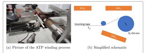
**Fig. 1** The ATP winding process with the three radiative heat sources marked as  $RHS_1$  and  $RHS_2$ , the incoming tape temperature is  $T_{in}$ , the cylindrical deposition base has a radius  $R_c = 54$  mm and a controlled temperature  $T_b$
