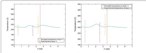
(a) Deposition of the third layer, l = 3, (b) Deposition of the fifth layer, l = 5, along along with the temperature measured by with the temperature measured by probes 1, probes 1, 2, 3 and 4 illustrated in figure 2(b) 2, 3 and 4 illustrated in figure 2(b) for set 1 for set 1 of experimental parameters of experimental parameters
