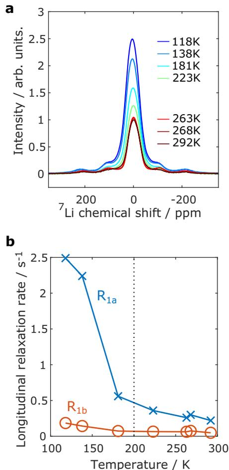
**Fig. 6** Solid-state NMR on  $\text{Li}_2\text{TiSe}_3$ . **a** Static  $^{7}\text{Li}$  spectra as a function of temperature. **b**  $^{7}\text{Li}$  longitudinal relaxation components  $R_{1a}$  and  $R_{1b}$  plotted against temperature.
