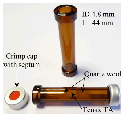
Fig. 2. Custom-built glass tube intended for packing with adsorbents and thermal desorption in the nCx-TD. ID = internal diameter, L = length.
