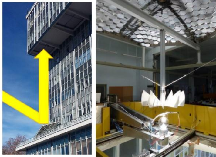
229 Figure 6: The two parts constituting the experimental device. On the left, the heliostat and the hatch and, on the right, the 230 OPTISOL test bench held by a mechanical arm (in grey) and the concentrator (above). The photographs were taken from 231 [16].
