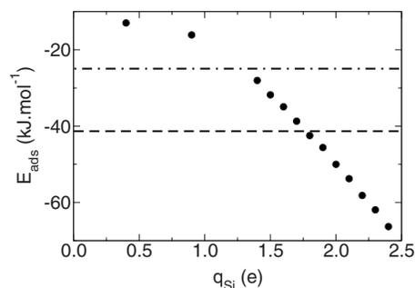
FIG. 1. Adsorption energy of SPC/E water in silicalite, as a function of the partial charge on silicon. The framework is hydrophobic for  $q_{Si} < 1.6$ . The dashed and the dot-dashed lines show, respectively, the vaporization enthalpy of the SPC/E model of water (Ref. 39) and the smallest experimental adsorption energy of water in silicalite (Ref. 6).
