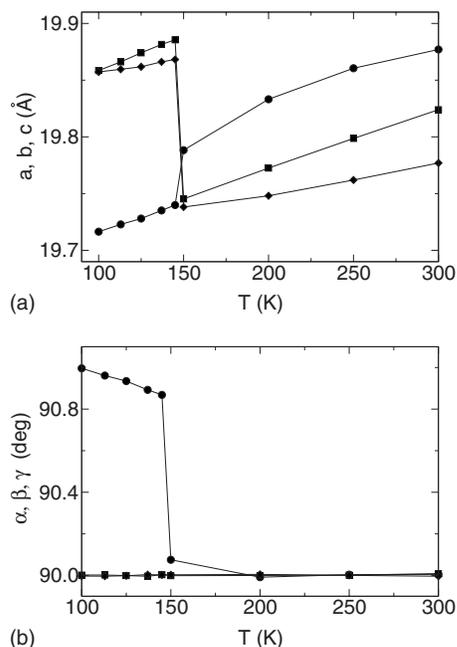
FIG. 4. Simulated monoclinic to orthorhombic transition of silicalite, BKS<sup>mod</sup> model: (a) Cell sides, shown for convenience of plotting as:  $a+0.3$  Å (■),  $b$  (●),  $c+6.5$  Å (◆); (b) cell angles:  $\alpha$  (■),  $\beta$  (●),  $\gamma$  (◆).
