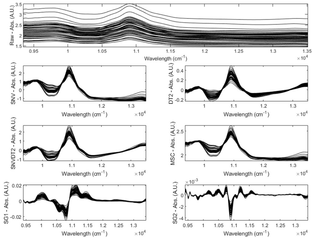
**Figure 3** Different preprocessing algorithms were applied to the raw spectra acquired with *MultiPurpose Analyzer I* (Bruker, USA). (a) Raw spectra; (b) SNV preprocessed spectra; (c) DT2 preprocessed spectra; (d) SNV + DT2 preprocessed spectra; (e) MSC preprocessed spectra; (f) SG1 preprocessed spectra; (g) SG2 preprocessed spectra.
