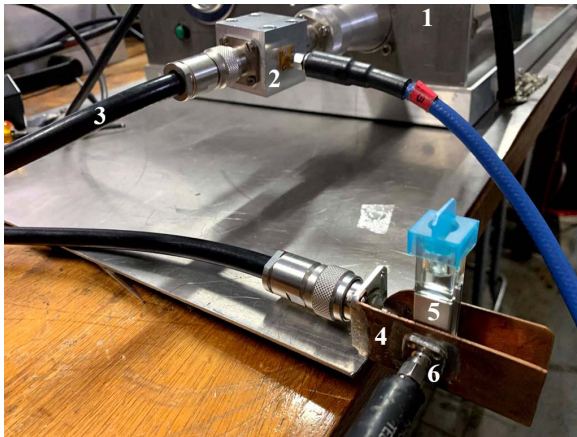
Fig. 2. Experimental arrangement for subnanosecond PEF processing. The numbers 1–6 represent the generator (1), capacitive voltage divider (main voltage probe) (2), RG214-U 50 \Omega coaxial cable (3), two parallel-plate electrodes (4), 4-mm electroperoration cuvette (5), and SMA-type V-dot probe (6).
