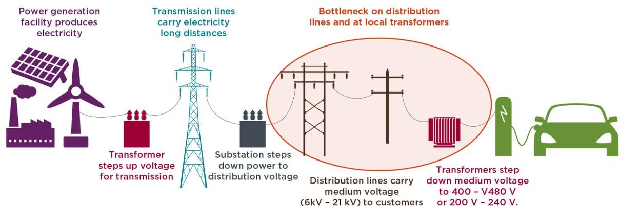
**Figure 1.** Schematic of the power grid distribution [1].
