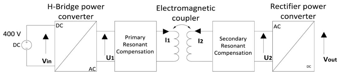
**Figure 2.** Block diagram of the power transmission system.
