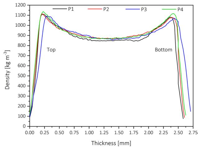
**Fig. 2** Vertical density profiles of the tested panels
