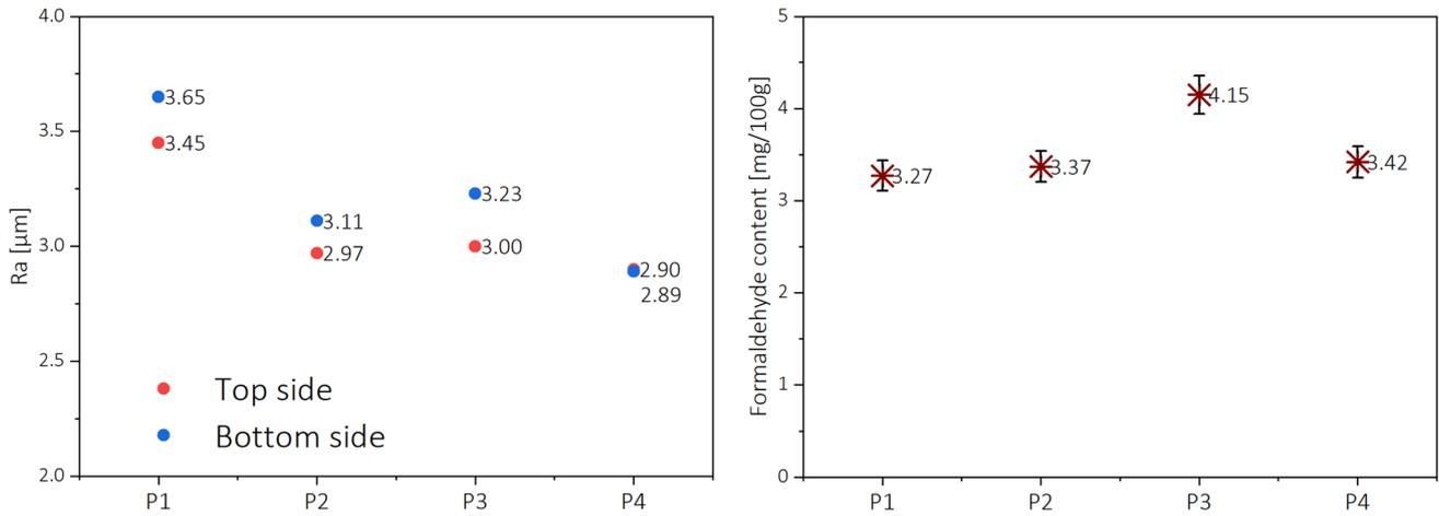
Fig. 6 Surface roughness and formaldehyde content
