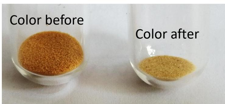
**Figure 6.** Change of color of the supported catalyst CAT D-ox after supercritical CO<sub>2</sub> extraction of Pd assisted by the copolymer P(4VP-*grad*-FDA) at 40 °C and 25 MPa: a) color of CAT D-ox before extraction; b) color CAT D-ox after extraction.
