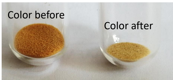
Figure 6. Change of color of the supported catalyst CAT D-ox after supercritical CO 2 extraction of Pd assisted by the copolymer P(4VP- grad -FDA) at 40 °C and 25 MPa: a) color of CAT D-ox before extraction; b) color CAT D-ox after extraction.
