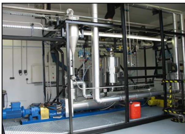
Figure 3—Photograph of the 165 bar hydrate loop.
